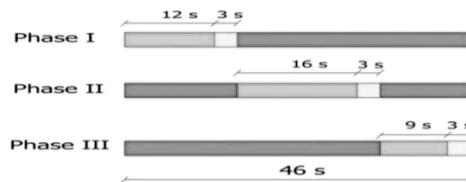
Fig. 12 - Optimized timing plan of the selected intersection
