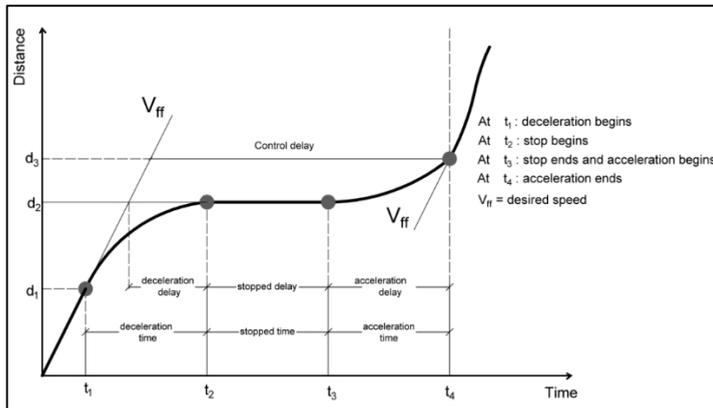
Fig. 4 - Diagram of intersection delay components [12]
