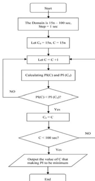
Fig. 6 - Flow chart for cycle time optimization [9]
