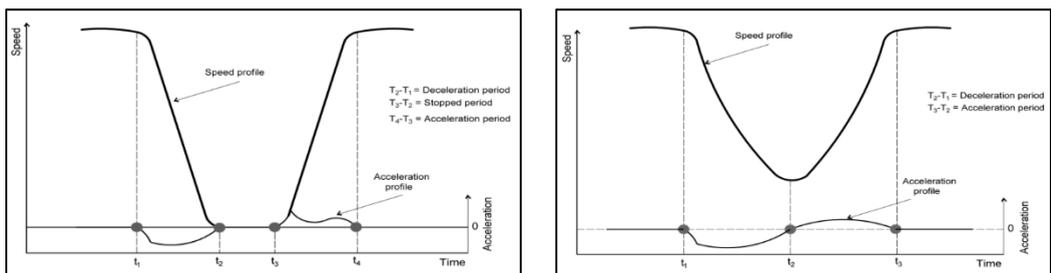
(a) Speed profile with stopped delay
