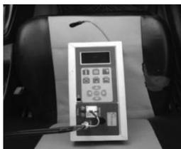
Fig. 1 - Gas analyzer instrument installed in a vehicle
