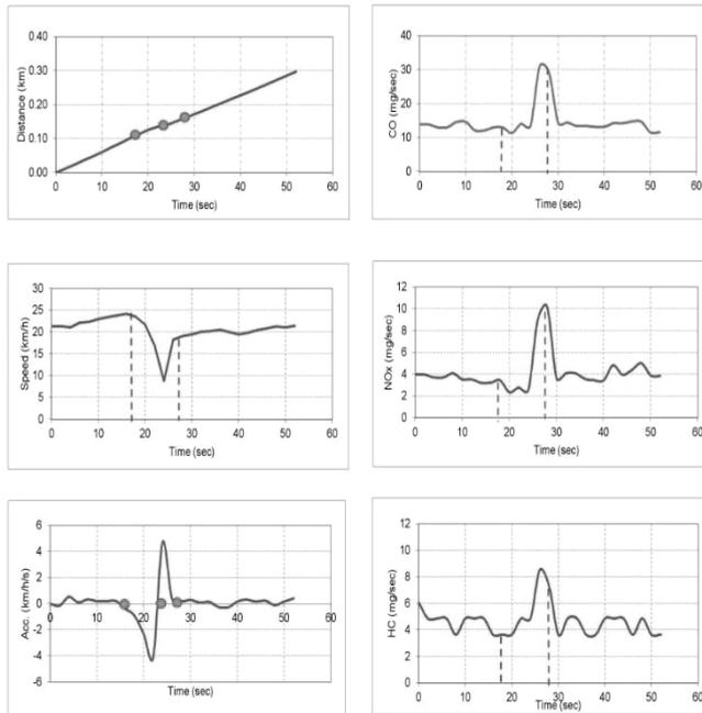
Fig. 9 - Example of speed profile, time–space diagram, acceleration profile and vehicle emissions without stopped delay for left-turn movement of eastbound direction at the selected intersection
