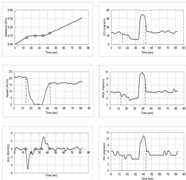
Fig. 10 - Example of speed profile, time–space diagram, acceleration profile and vehicle emissions with stopped delay for left-turn movement of eastbound direction at the selected intersection
